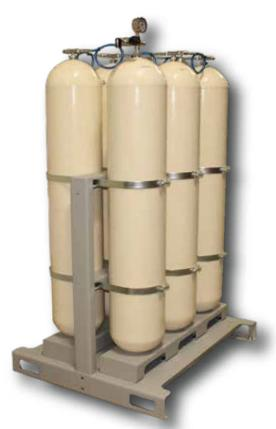
In contrast, ASME Cylinders do not require recertification. The dry weight of the ASME Cylinder is 400 lbs., and it is rated at 491 cf @ 6000 psi. Certified ASME Relief Valve is a requisite for ASME Cylinders.
